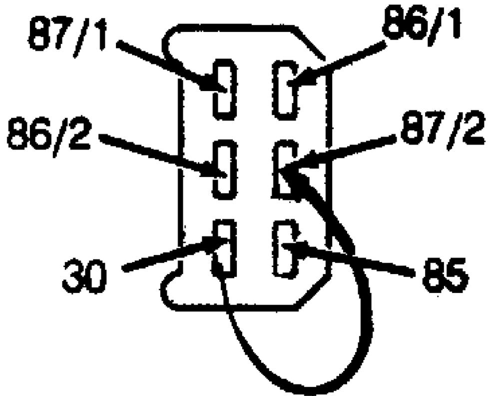
Fig. 3: Identifying Fuel Injection System Relay Terminals (940)
